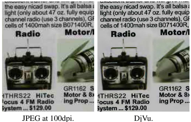
Figure 1. Comparison of JPEG at 100dpi (left) with quality factor 30% and DjVu (right). The file sizes for the complete pages are 82 KB for JPEG and 67 KB for DjVu
