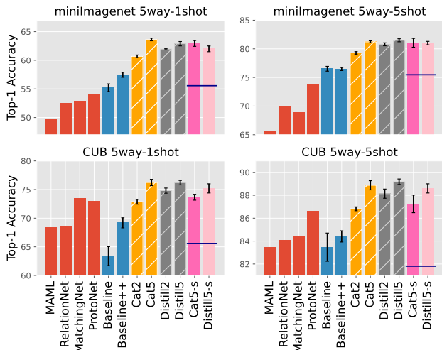
Figure 6. Few-shot learning performance on MINIIMAGENET and CUB. Four common few-shot learning algorithms are shown in red (results from Chen et al. (2019)). Two supervised transfer methods, with either a linear classifier (BASELINE) or cosine-based classifier (BASELINE++) are shown in blue. The DISTILL and CAT results, with a cosine-base classifier, are respectively shown in orange and gray. The CAT5-S and DISTILL5-S results were obtained using five snapshots taken during a single training episode with a relatively high step size. The dark blue line shows the best individual snapshot. Standard deviations over five repeats are reported.
