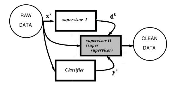
Figure 4: Block diagram of the cleaning scheme: super-supervision.
