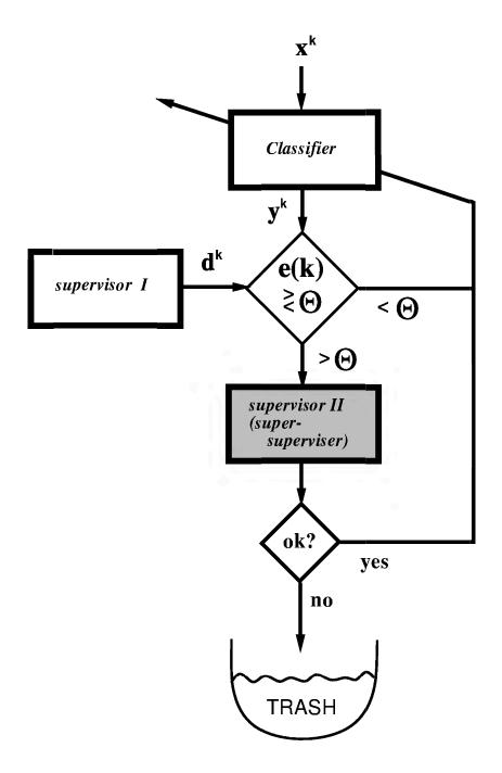
Figure 5: Flow diagram of the interactive version of the cleaning scheme.
