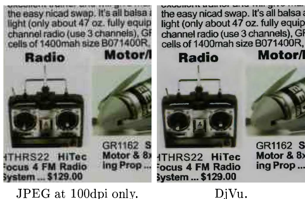
Figure 4: Comparison of JPEG at 100dpi (left) with quality factor 30% and DjVu (right). The images are cropped from hobby002 . The file sizes are 82K for JPEG and 67K for DjVu
